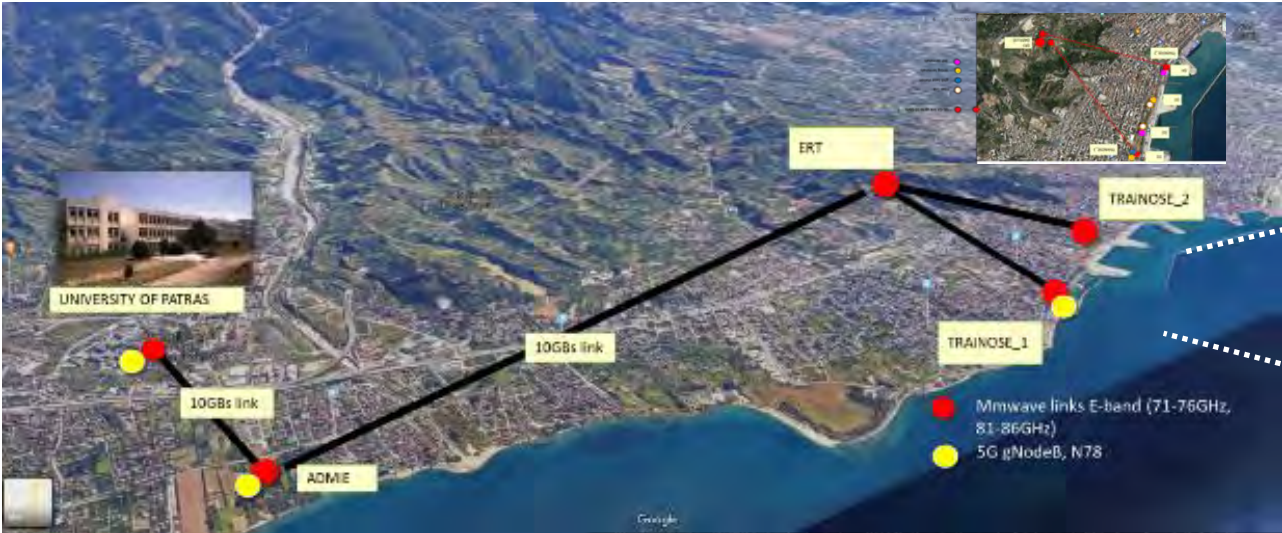
Figure 6-4 Patras Facility area and sites. The area between points TRAINOSE_1 and TRAINOSE_2 is enlarged in Figure 6-1
