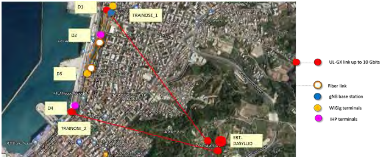
Figure 6-1 Network diagram for UC #1.1 over Patras satellite map
