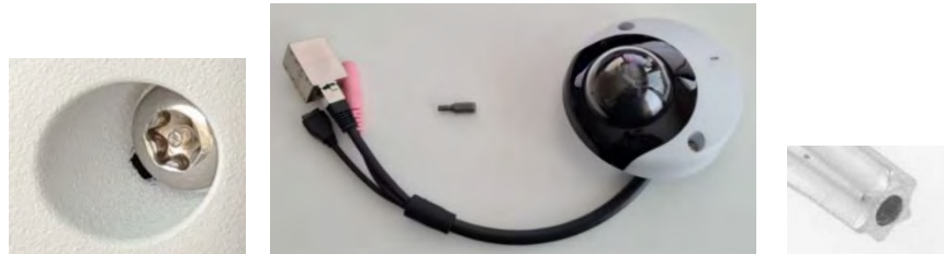
Figure 3-22 Rail Critical Services – CCTV Streaming – Network camera Axis P3935-LR – front side
