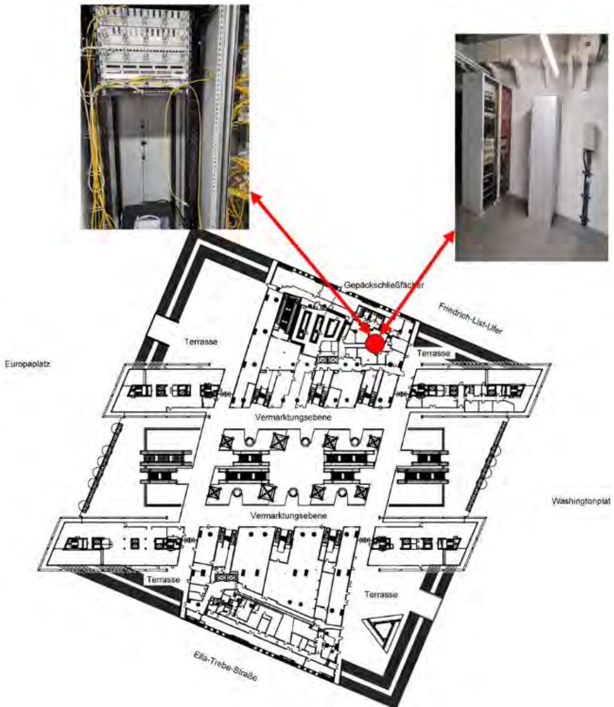
Figure 3-6 Equipment Office location at ground level, server room and rack space
