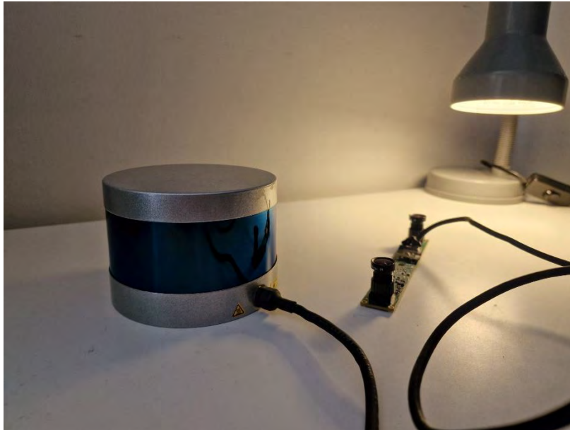
Figure 4-26 Cylindrical shape is the Lidar, the pair of oculars is the stereo camera
