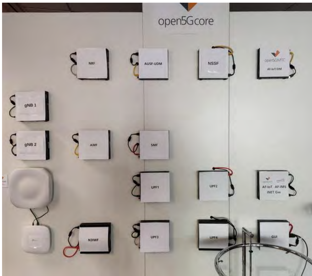
Figure 5-8 Open5GCore station and its components in lab
