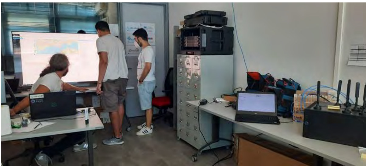
Figure 3-13 Lab tests of UiTOP platform. The laptop shown here operates as an industrial sensor connected to the platform through 5G.
