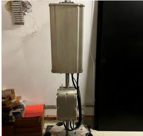
Figure 6-6 5G SA deployment in LAB environment
