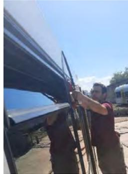
2<sup>nd</sup> mmWave roof top antenna+ sub 6 antenna
