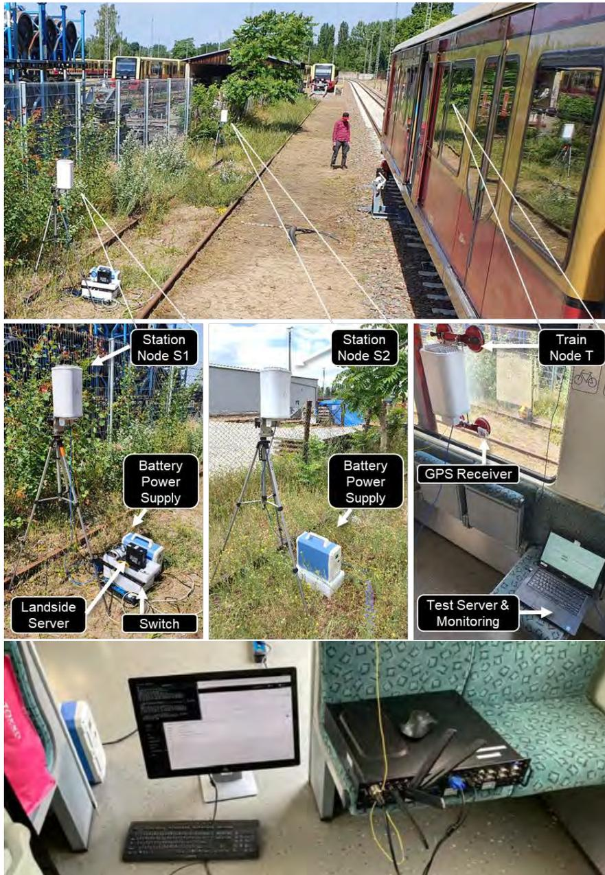
Figure 3-46 Overview of the system setup for the *Berlin-Schöneeweide* field trial: a) View of the station node S1, b) View of the station node S2, c) View of the train node T e) the railSTACK server on the train
