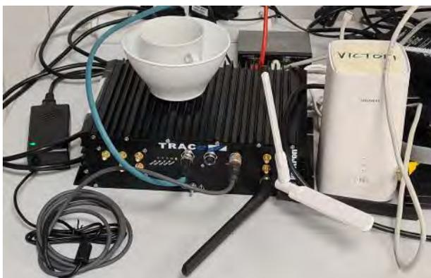
Figure 3-24 5G mobile gateways: KCC 5G GW (black unit) and Huawei CPE Pro 2 (white unit).
