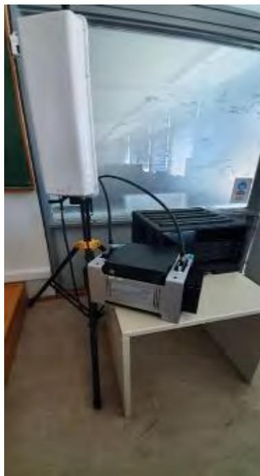
Figure 4-48 The gNodeB that was used in the lab tests and will be used in the field trials connected to the stanchion
