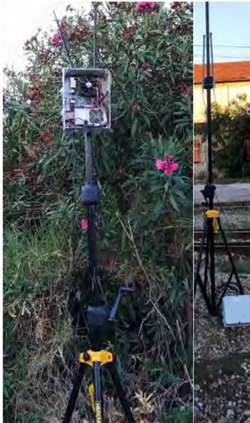
Figure 4-19 Sub-6 GHz track-side nodes mounted with different types of antennas
