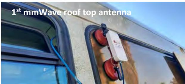
1<sup>st</sup> mmWave roof top antenna
