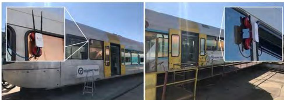
Figure 4-22 Overview of the mmWave train-mounted nodes T1 (right) and T2 (left)
