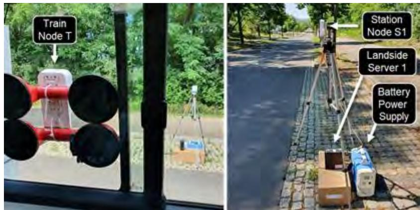
Figure 4-8 Overview of the system setup for the IHP lab trial: a) View of the train node T, b) View of the station node S1
