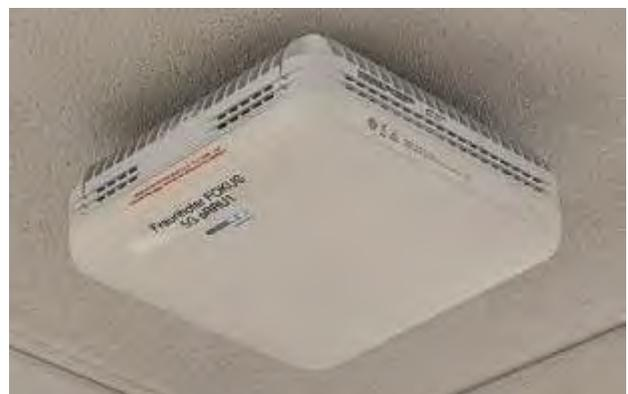
Figure 3-25 5G base station remote radio unit – FhG 5G pRRU1
