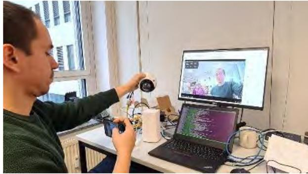
Figure 3-16 The CCTV camera internal processing and coding gives a delay of around 300 ms
